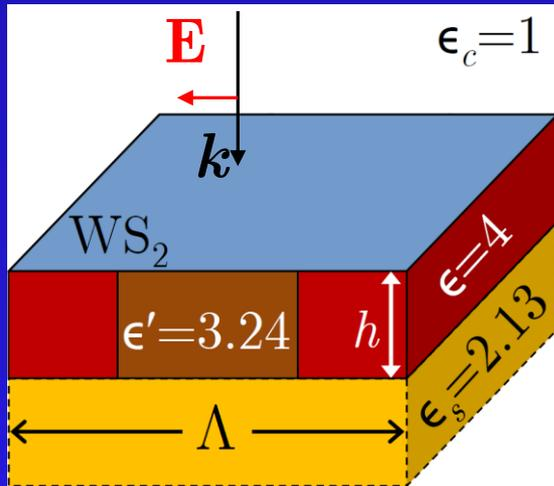
Textured slab waveguide + TMDC monolayer
