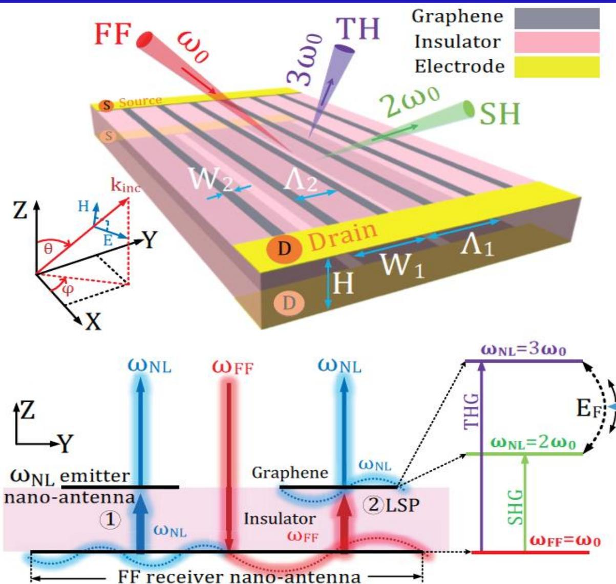
Fundamental plasmon at FF: efficient light in-coupling
