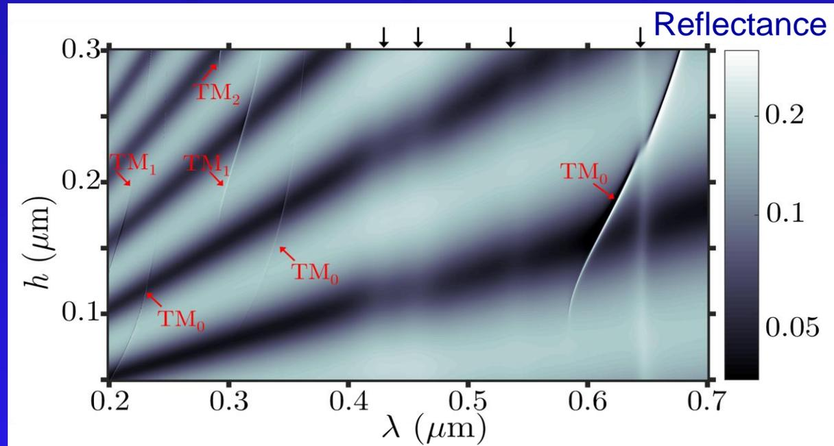
Textured slab waveguide + TMDC monolayer
