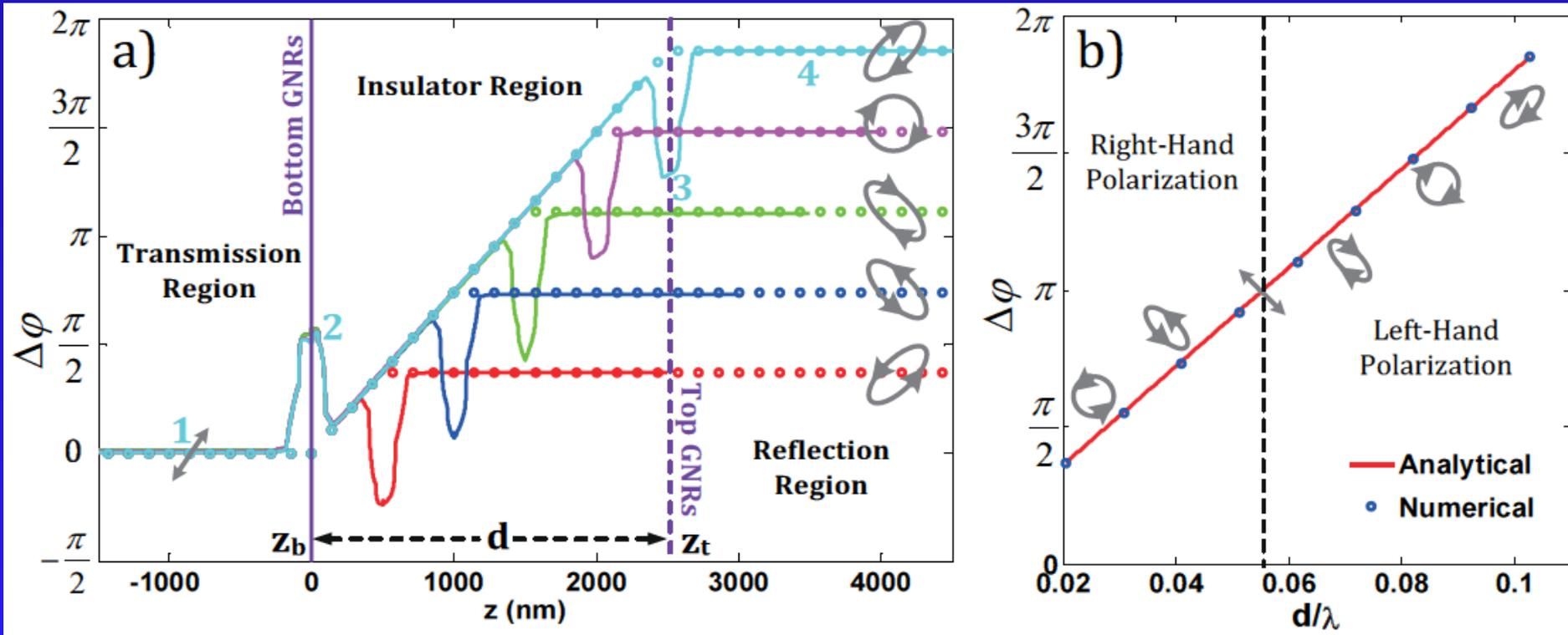
$$\Delta\phi = \frac{4\pi n d}{\Lambda} \quad \Lambda = \frac{\lambda}{m} = \frac{\lambda}{3} \quad \text{TH wavelength}$$
