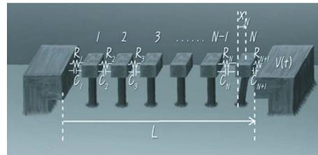
FIG. 1. (Color online) Sketch of  $N$  coupled nanoelectromechanical shuttles.
