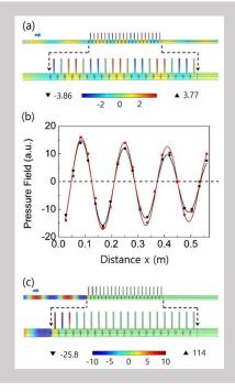
Realization of unidirectional zero reflection based on a loss-gain balanced metamaterial
