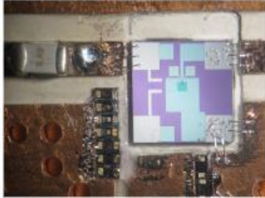
Niobium SQUID amplifier made by Sean O'Kelley Clarke Lab, Berkeley
